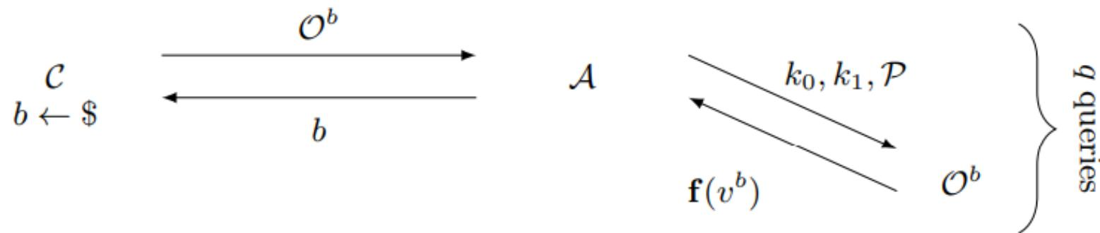
Figure 1: The privacy model for the glitch-extended  $t$ -threshold-probing security consisting of a challenger  $\mathcal{C}$ , an adversary  $\mathcal{A}$ , a left-right oracle  $\mathcal{O}^b$ , two inputs  $k_0, k_1$ , a set of probes  $\mathcal{P}$ , and a noisy leakage function  $\mathbf{f}(v^b)$  of the probed wire values  $v^b$  in the circuit  $C(k_b)$ .
