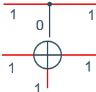
node works as XOR-gate for any 2 inputs;
